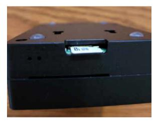
Be careful when installing the SD card. It is possible to insert the card between the case and the card slot instead of getting it into the slot. If that happens, you will need to unscrew the four screws on the back to open the housing and retrieve the SD card.
