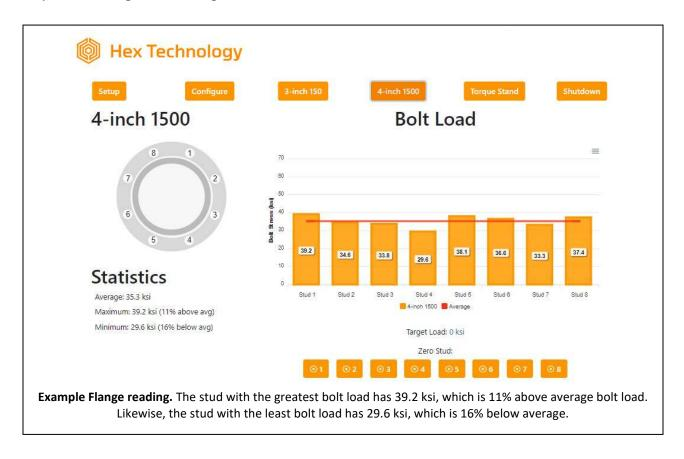
The load on each stud appears as a bar with a number indicating the bolt load value inside.
