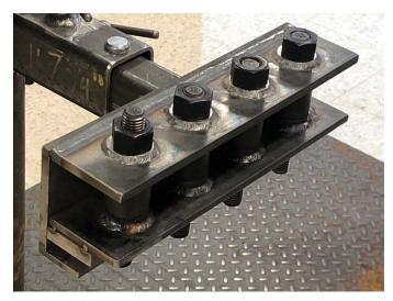
The torque stand allows you to record up to 5 trials in a single test.
