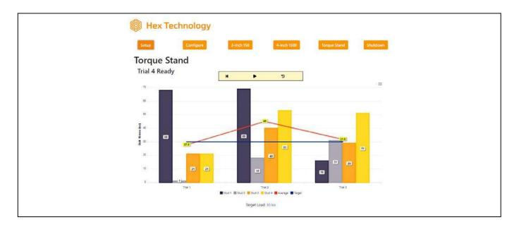
Once you have finished applying torque to all studs, press the pause ( II ) button to save the values measured within that trial.
