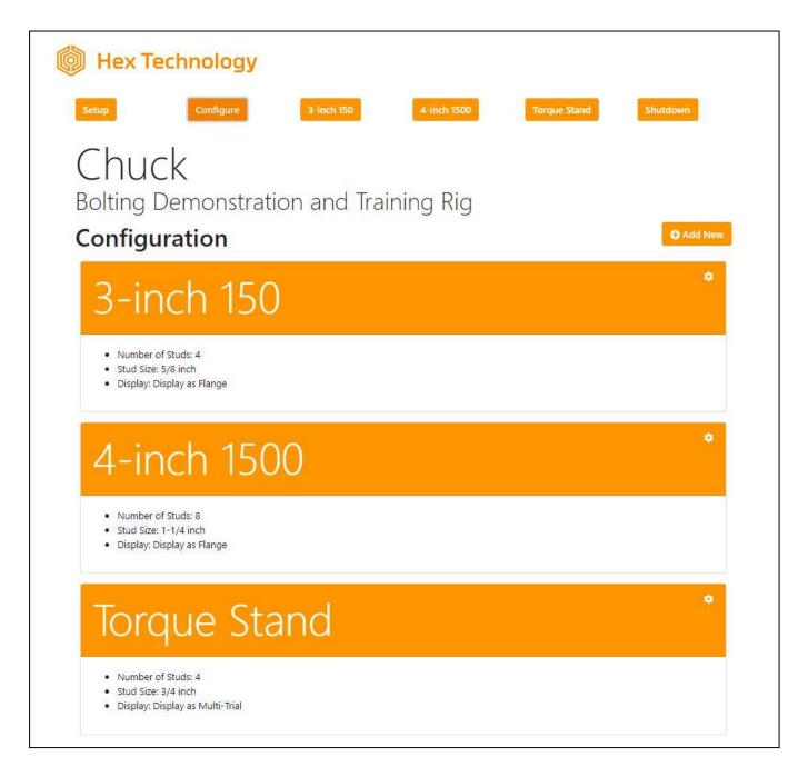
You can configure your system to measure bolt load on multiple flange assemblies. Those assemblies are called "Stations."
